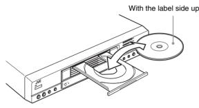
• To insert an 8-cm disc, place it in the inner recess.
